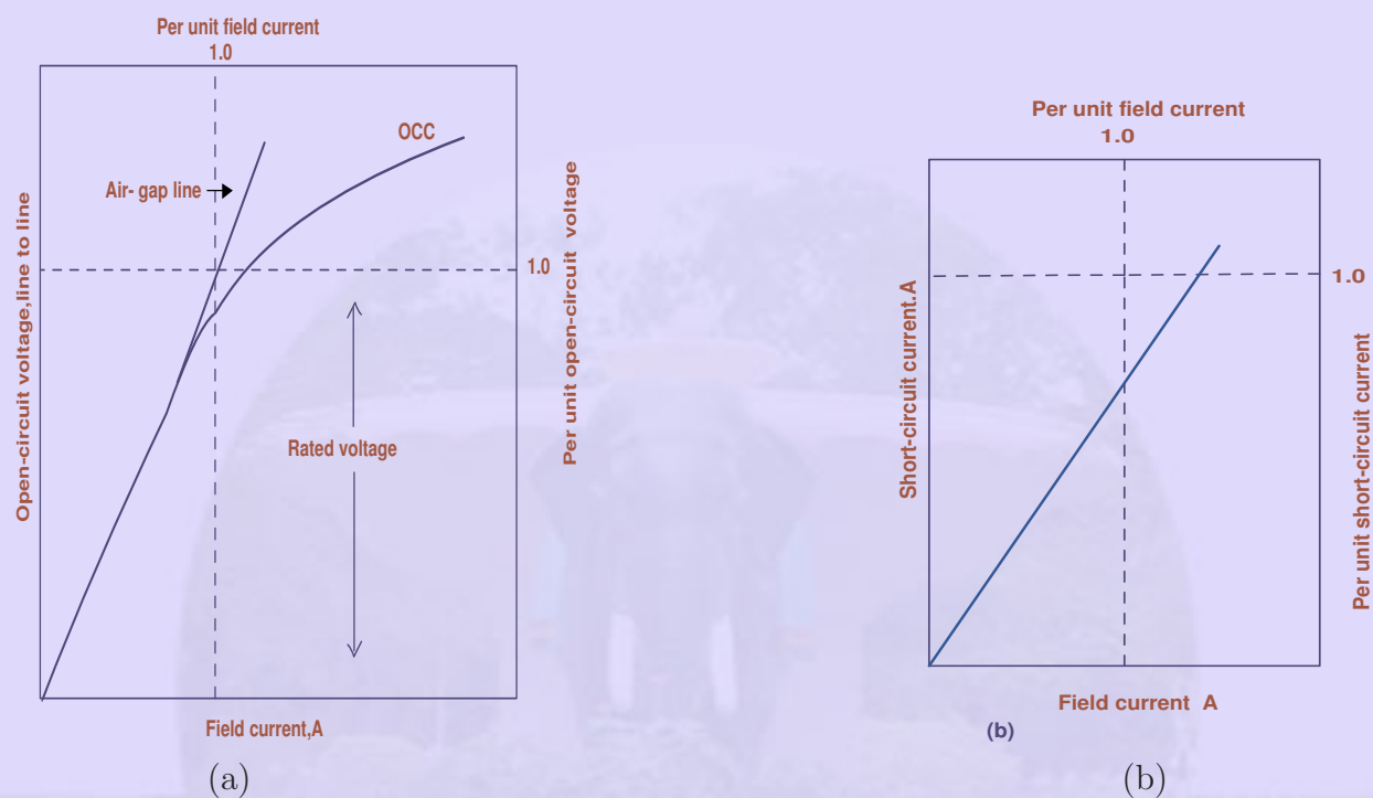
Figure 27: (a) Open circuit characteristic and (b) Short-circuit characteristic
